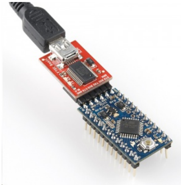
FTDI Basic programming a Pro Mini. Note RX and TX's crossed!
